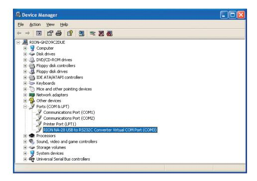
The indication "RION NA-28 USB to RS232C Converter Virtual COM Port" should be shown as COM port name. If this is not shown, check the connection between the NA-28 and the computer (step 1). If there is an "x" over the icon, the port is not functioning normally. Install the driver again.
